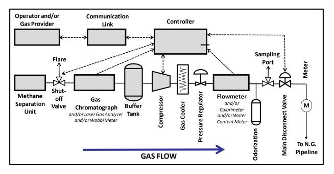
Figure 2. Generic Biomethane Interconnection Components
