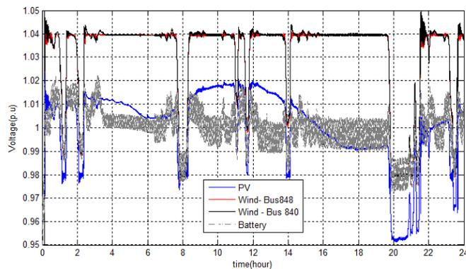
*Voltages at renewable source buses in grid connected mode.*
