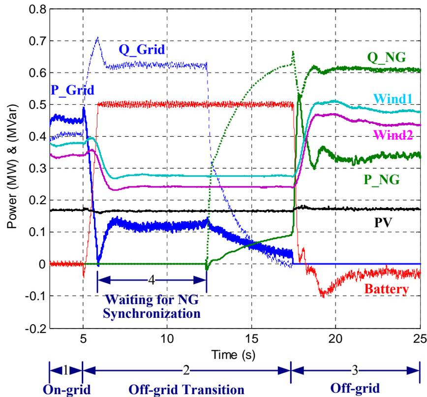
*Intentional islanding: real and reactive power delivered by the grid and five sources with minimum load and maximum renewables.*
