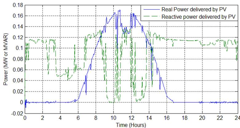
*Active and reactive power delivered by 0.25MW solar PV.*
