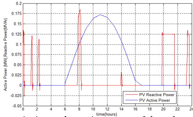
*Active and reactive power of the solar PV in grid connected mode.*
