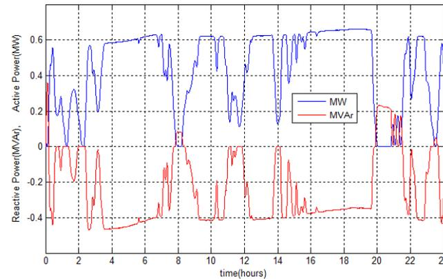
*Active and reactive power of the wind turbine on bus 840 in grid connected mode.*
