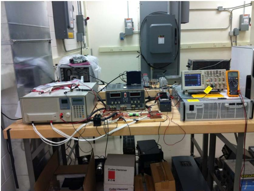
**Battery cell test setup.**
