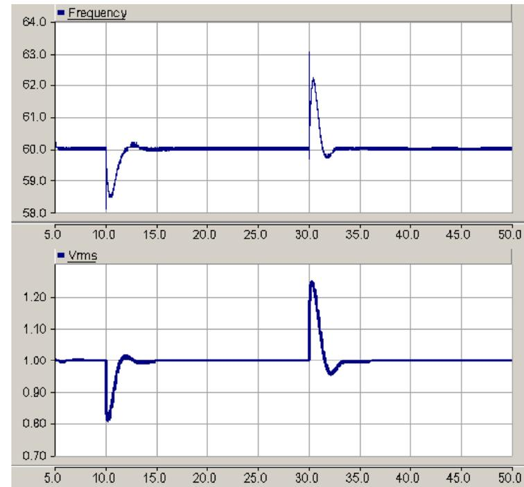
*Simulation results for the diesel generator when load steps are applied at 10s and 20s.*
