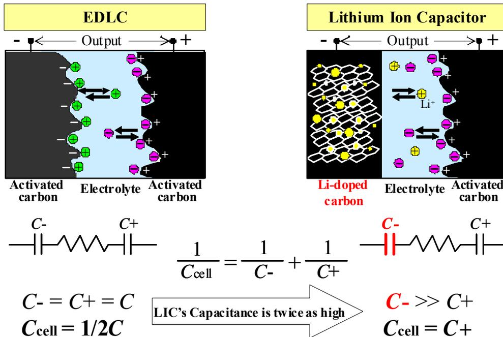
Concept of Lithium-ion Capacitor.
