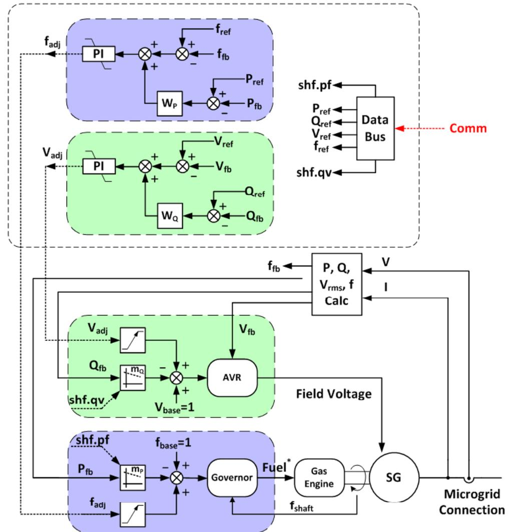
*The block diagram of the controls for voltage and frequency of the diesel generator.*
