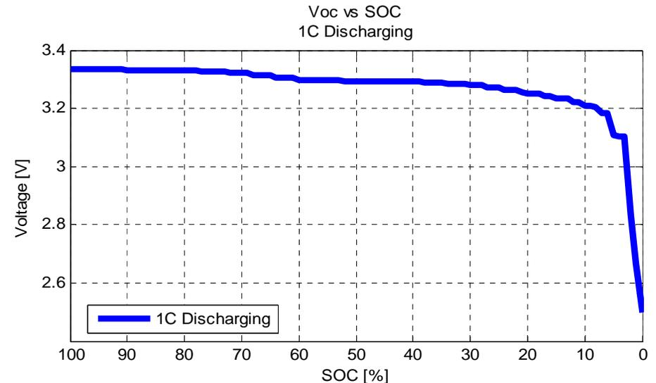
Battery vs. SOC traces at various discharging currents.
