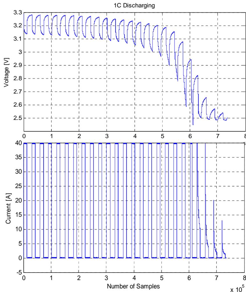
Voltage and current traces for battery discharging voltage (above) and current (below).
