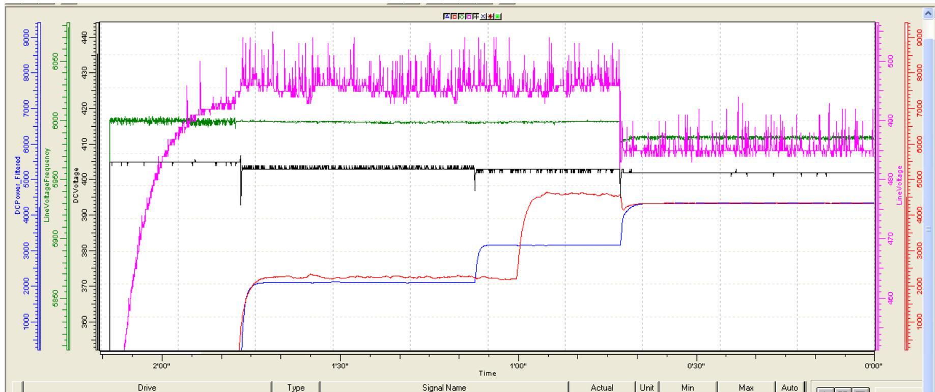
*Output voltage, frequency, power, and DC bus voltage in grid-tie and island modes.*
