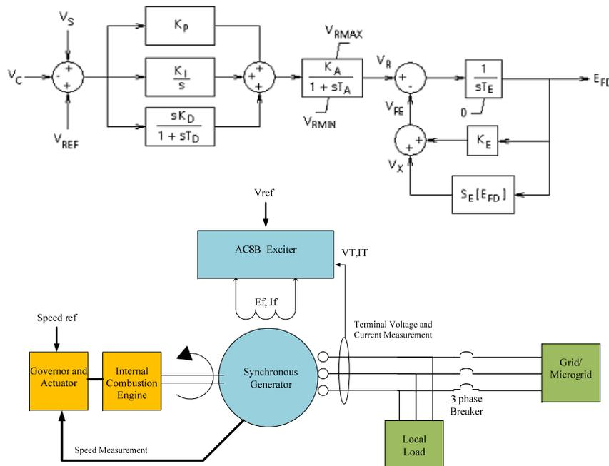
*Basic block diagram of an NG generator connected to a grid/microgrid.*
