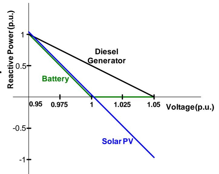
*The reactive power droop mechanism for diesel generator, solar PV and battery in the microgrid.*
