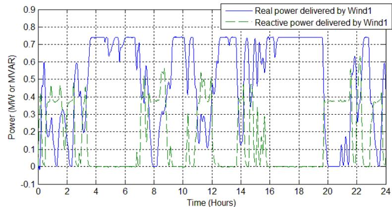
*Active and reactive power delivered by one of the 0.75MW wind turbines.*
