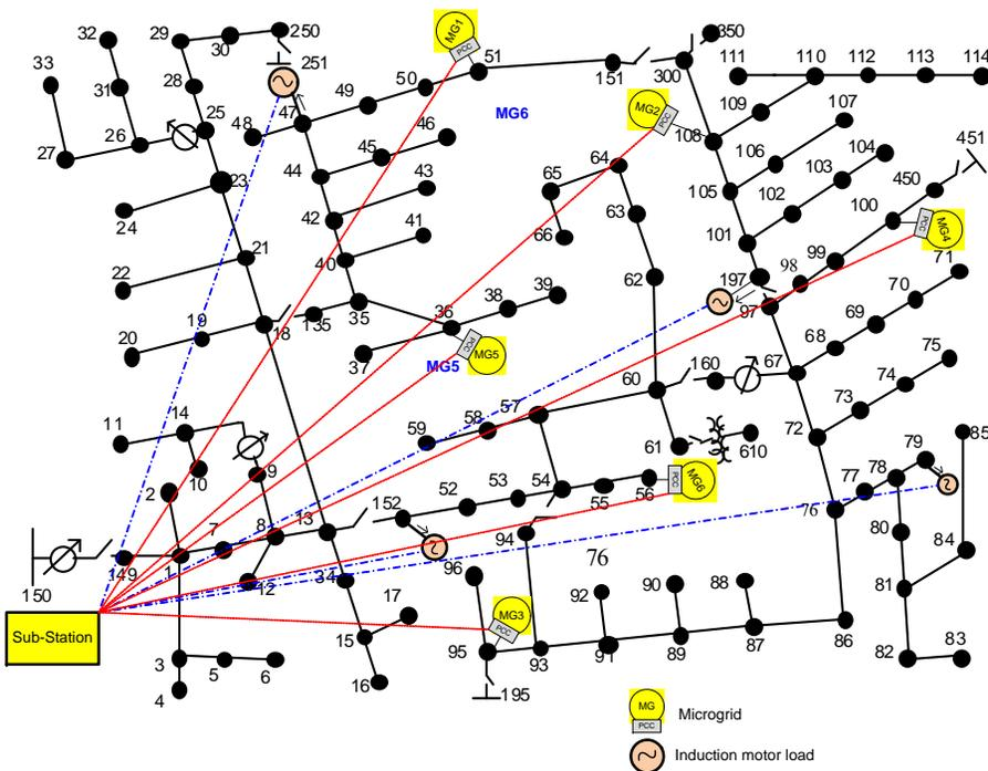
*Configuration of the IEEE 123 bus test feeder with microgrids.*
