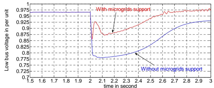
*Bus voltage profile with and without microgrids support during induction machine starting.*
