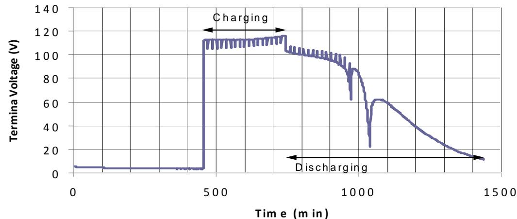
**Testing and modeling of Zinc Bromide battery. Components in the model are non-linear functions of SOC and temperature.**
