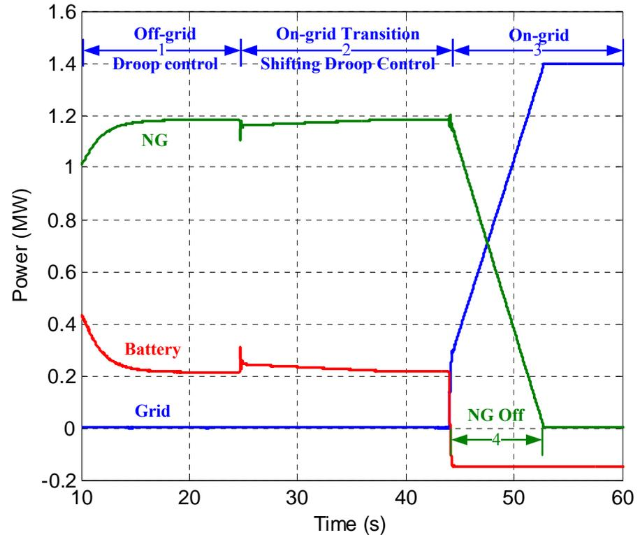
*Waveforms of power delivered by grid, natural gas generator and battery during reconnection.*
