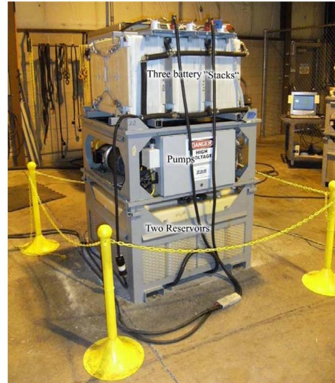
Stack Assembly and electrolyte flow in a Zinc-Bromide energy storage system.
