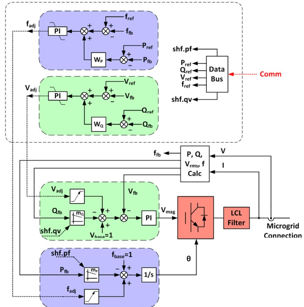
*The block diagram of the controls for voltage and frequency of storage inverter.*
