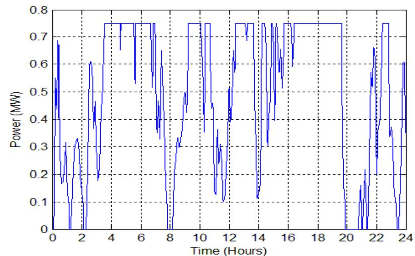
*The power profile of a 250kW solar PV plant and 750kW wind turbine.*
