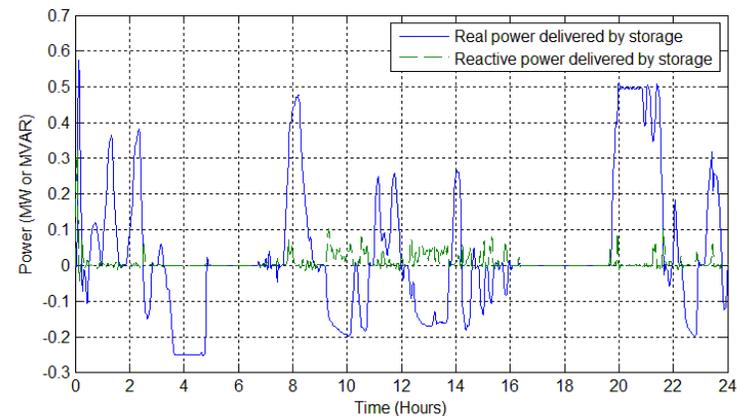
*Total active and reactive power delivered by two 0.25MW battery storage systems.*
