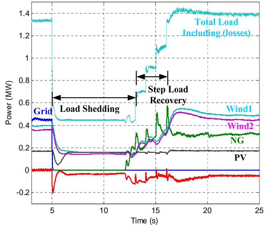
*Unintentional islanding: total load and real power delivered by grid and five sources with minimum load and maximum renewables.*
