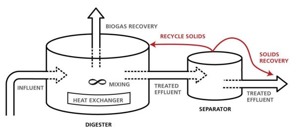
Figure 4 - Simplified anaerobic contact process schematic
