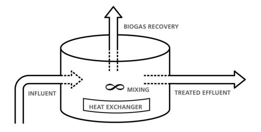
Figure 3 – Simplified complete mix digester schematic
